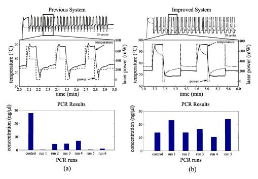
**Figure 1**: Laser power, microchip temperature profile, and amplification efficiency in the open-loop, rapid, laser PCR system (a) before and (b) after implementation of pressure and temperature controlled environment, oil encapsulation, and laser power optimization.
