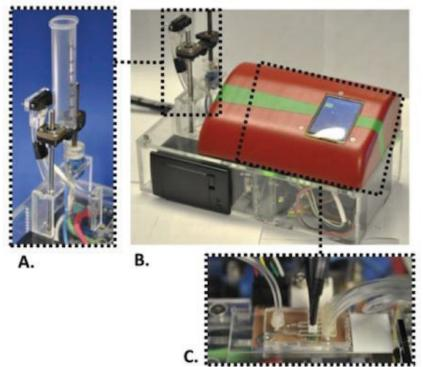
**Conclusion:** The system enables real-time testing of human whole blood for shear induced platelet thrombosis at multiple shear flow conditions. The size and ease-of-use of the system allows for Point-of-Care measurements of high shear clotting potential from individual patient blood samples. Future work will adapt this system for simultaneous treatments by different anti-platelet agents at varying dosages.
