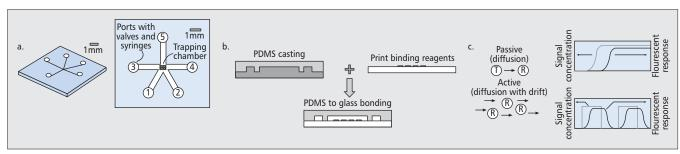
**Figure 3.** *a)* A multilayer microfluidic device that can be designed to allow input/output ports to deliver reagents, waste, and cells to a trapping chamber; b) fabrication steps of the device; and c) stimulation and measurement of the response of the cells to both constant and time varying molecular signaling conditions in either a passive or active diffusion.
