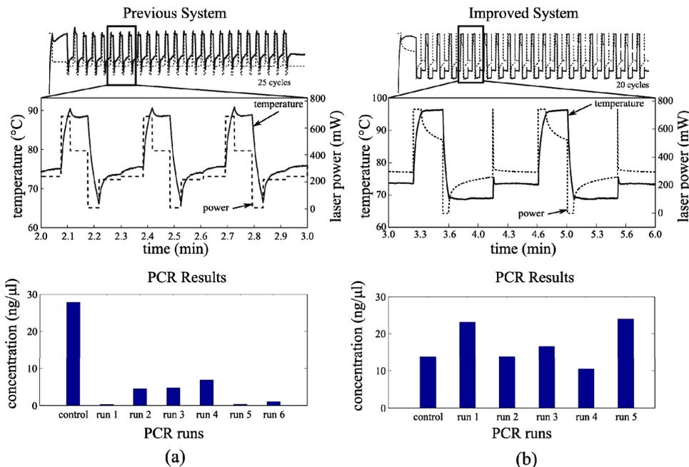
**Figure 1:** Laser power, microchip temperature profile, and amplification efficiency in the open-loop, rapid, laser PCR system (a) before and (b) after implementation of pressure and temperature controlled environment, oil encapsulation, and laser power optimization.
