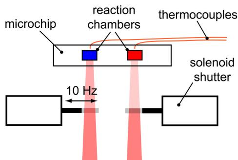
*FIGURE 3. Infrared laser sources and solenoid shutters can be used with closed-loop control to perform PCR on multiple distinct targets simultaneously by monitoring temperature and independently modulating the laser beams.*
