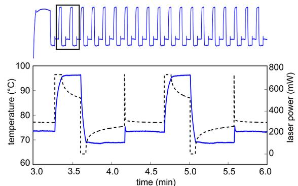
**FIGURE 2.** Using a calibration of laser power and reaction temperature combined with heat transfer modeling, an optimized laser power profile (dashed line) was generated for open-loop thermocycling.
