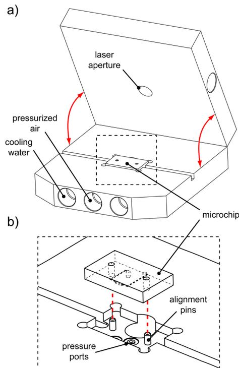
**FIGURE 1.** The environmental control fixture provides a mechanically and thermally repeatable environment for the microchip (inset) while allowing microscope and laser access to the PCR sample contained in a chamber in the center of the microchip.
