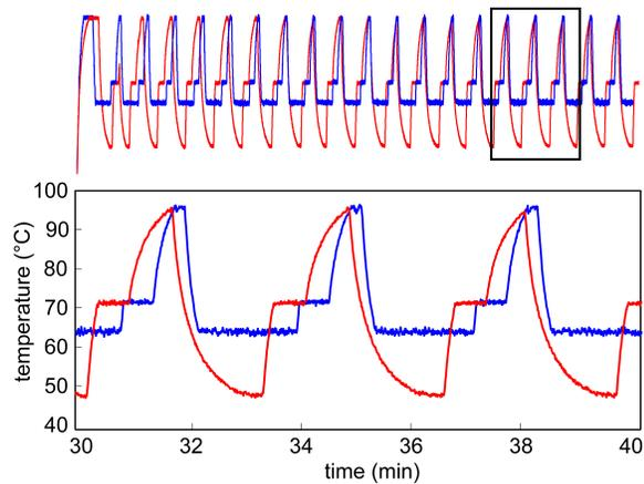
**FIGURE 4.** Closed-loop control and optical modulation enable independent temperature profiles for amplifying multiple genetic targets in a single instrument run.
