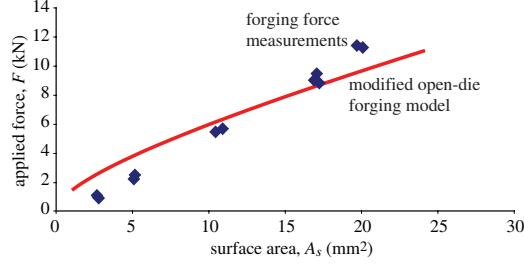
**Figure 2.** Forging force theory and experimental measurements vs. molded surface area.
