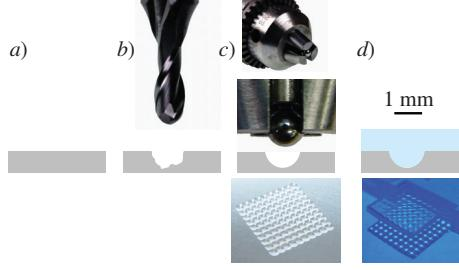
**Figure 1.** Schematic of lens array mold manufacturing process and photographs of a 100 lens array mold and molded part. *a)* A blank aluminum mold is faced and polished. *b)* A rotating ball-end mill is used to cut an array of divots. *c)* A tungsten-carbide sphere is lowered onto the surface to deform the divots to the final shape. *d)* The mold is used to injection mold lens arrays, as we have done for arrays containing over 10,000 lenses.
